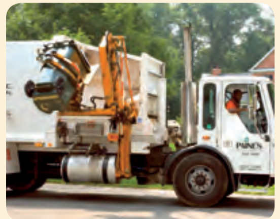
emptying by side loader with clamp lift
