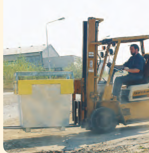
▲ Transport by forklift truck – by means of standard size pockets mounted on the base
