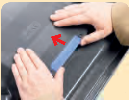
Fitting and removal of the “ ergolid clip ”
