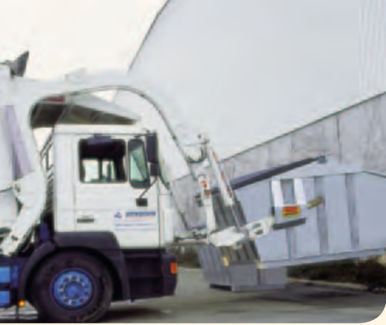
◀ Front loading 5.0 m 3 container in service
