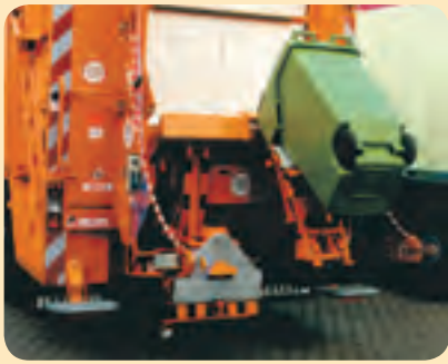
rear loader with combined comb/diamond-lifter
