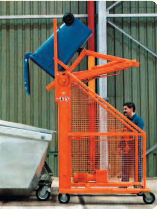
▲ The Schuettomat emptying a refuse bin into a large container
