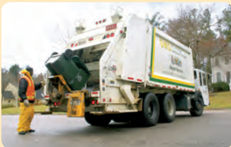
emptying with standard bar-lock system
