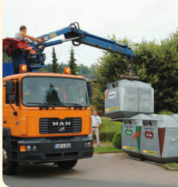
Glass collection, special discharging system
